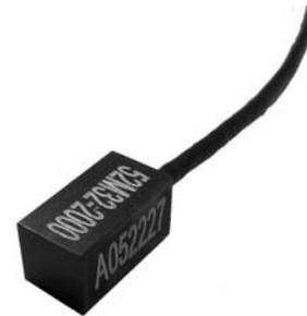
The **Model 52M32** accelerometer has an advanced piezoresistive MEMS sensing element which offers excellent dynamic range and stability. This unit features a full bridge output with an operating temperature range from -40 to +90°C. A slight amount of gas damping provides outstanding shock survivability and a flat amplitude response to 6kHz.
